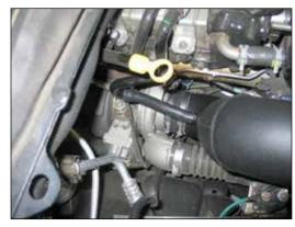
34. Install the provided air injection hose onto the air injection tube and then connect the open end to the 1/4"npt fitting in the K&N entry intake tube.
