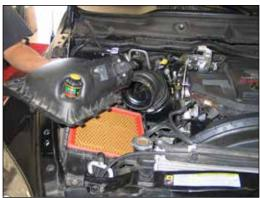
6. Remove the upper air box housing from the lower air box housing.
