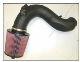
32. Install the K&N $^{\circledR}$  Air Filter onto the intake tube and secure with the provided hose clamp. NOTE: The filter is a tight fit, be sure the tube bead seats into the receiver groove in the filter.
