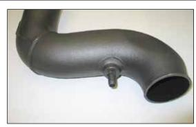
26. Install the provided  $\frac{1}{4}$ "npt fitting into the intake tube as shown.
